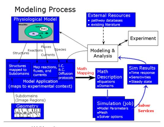
Abbildung 2: Modeling Process performed in Virtual Cell
